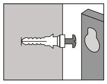
Line up screw with the round opening of the keyhole slot, then slide artwork down so screwhead is locked into place.
