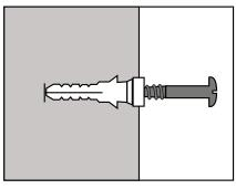
Insert screw into anchor leaving a minimum of 5/16 of mounting screw exposed from wall.
