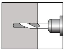
Using the drill bit size recommended on your wall anchor hardware, (not included) drill a hole equal to the depth of your anchor.
